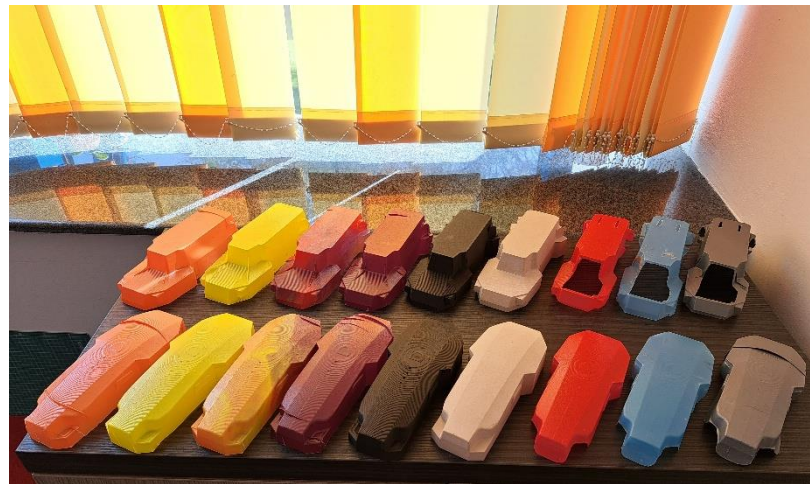
Figure 5. Thermoformed multi-colored casings, along with the molds and the 3 covers previously placed onto the drone
