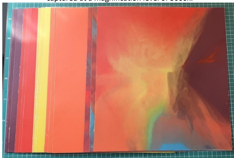
Figure 3. Plates/sheets processed by compounding/thermal pressing used for thermoforming covers made in various color combinations
