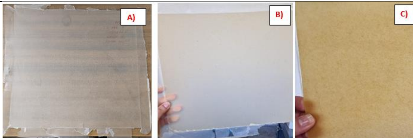
Figure 7. Plates obtained by compression method: A) PLA, B) PLA/untreated wool fibers and C) PLA/keratin
