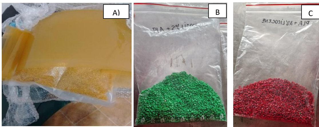
Figure 1. Samples of flame-retardant PLA in the form of granules and sheet (A) respectively granules obtained by extrusion-granulation based on PLA modified with additives and dyes (images B and C)
