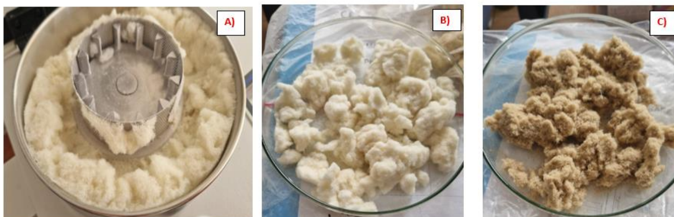
Figure 8. Turcana and Merino wool fibers treated with stearic acid (images A and B) respectively wool fibers treated with Savinase/APTMS
